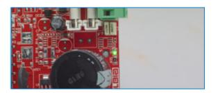
LED lights to indicate: power supply ON (green), actuator working conditions (yellow) and fault (red).
