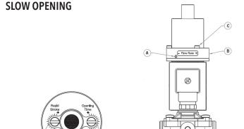
1. Flow rate adjustment. Loosen screw A and rotate cylinder B to the desired position. Tighten screw A to fix the position.
